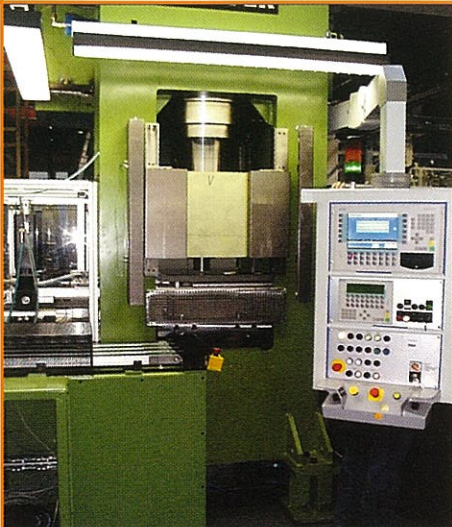
RPS 250: Sizing press with transfer, separator and deposit unit
